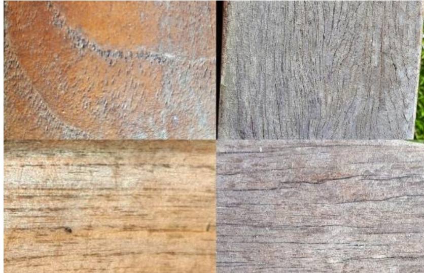
Figure 3. Material: Exterior Oil (to be used outdoor for basic treatment and maintenance of new and previously oiled wood surfaces such as decks, garden furniture) in the picture: to the left – with 2% of the multifunctional organoclay; to the right – without the multifunctional onal organoclay additive. Test description: previously oiled garden furniture 4 years old, oiled with/without 2% additive, 16-month outdoor exposure, Latvia
