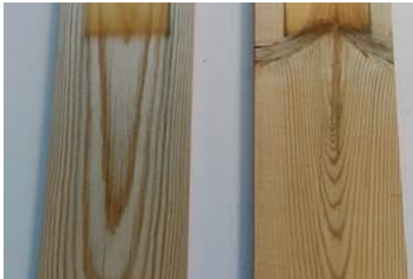
Figure 4. Material: standard decking oil in the picture: to the left – without the multifunctional organoclay; to the right – with 4% of the multifunctional additive. Test description: 7-month outdoor exposure, test method close to standard EN927-3, Denmark –West
