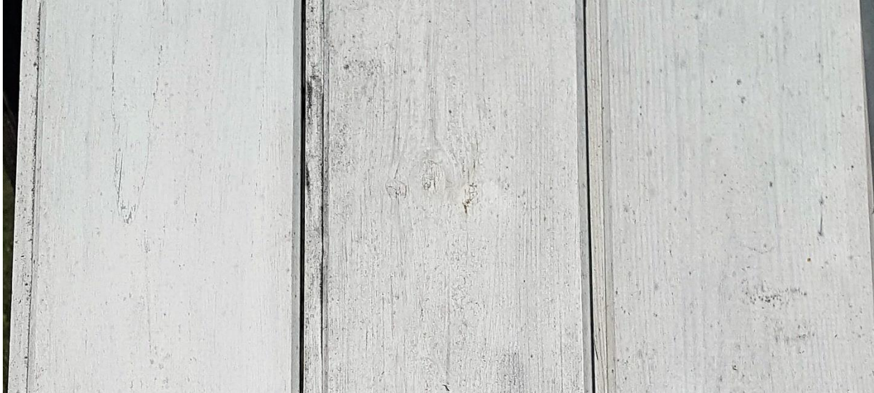
Figure 5. Material: White linseed oil paint in the picture: to the left – with 2% of the multifunctional organoclay additive; in the middle – without the multifunctional organoclay additive; to the right – with the 1% of the biocide PREVENTOL MP700. Test description: 12-month outdoor exposure, test method close to standard EN927-3, Latvia
